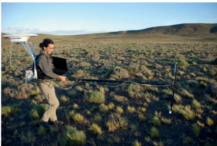
Fig.1. Surveying system where NEWTON first prototype will be integrated.
