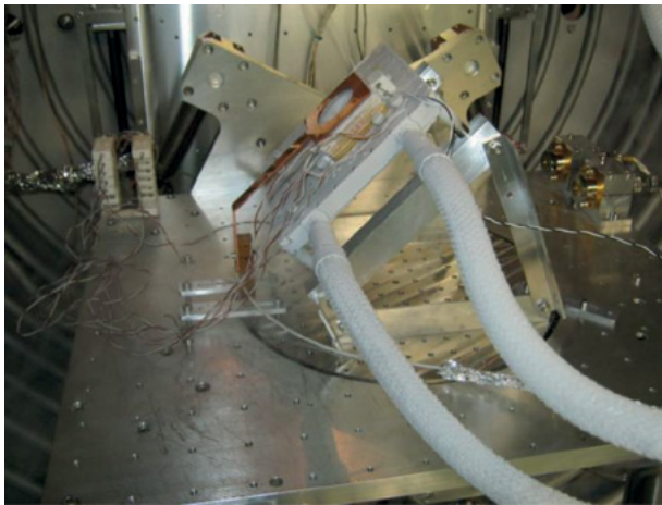
Fig. 2. Sample holder for regolith ice (with Cu ring) mounted on cryogenic stage, for ion irradiation experiments.
